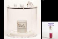
Figure 2. Method 1 - Calibration with Rad-Qual's X-Cal system being co-developed with author (PK). The system has <sup>68</sup>Ge/<sup>68</sup>Ga NIST traceable scanner, dose calibrator, and well counter sister sources.
