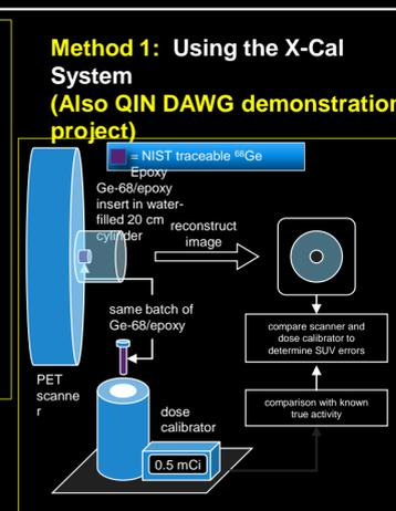
Figure 5. X-Cal Calibration.
