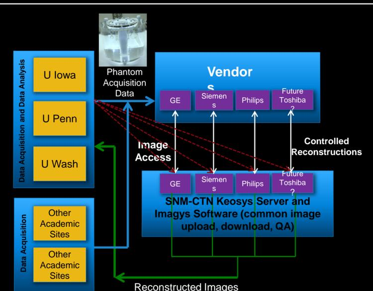
Figure 7. Acquisition, reconstruction and analysis workflow
