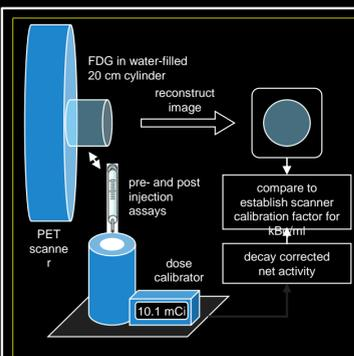
Figure 4. Standard calibration procedure
