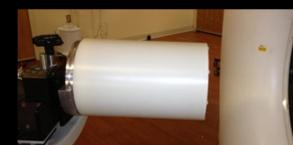
Figure 3. Method 2 - Calibration with 20 cm diameter, 30 cm length implicitly traceable <sup>68</sup>Ge/<sup>68</sup>Ga cylindrical phantom.
