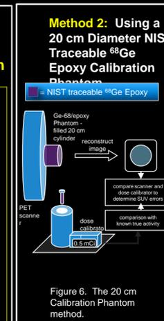
Figure 6. The 20 cm Calibration Phantom method.
